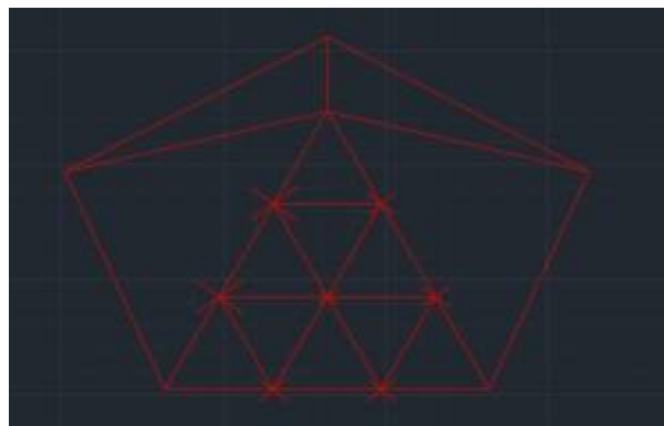
Figure 36: One face of the icosahedron divided in parts
