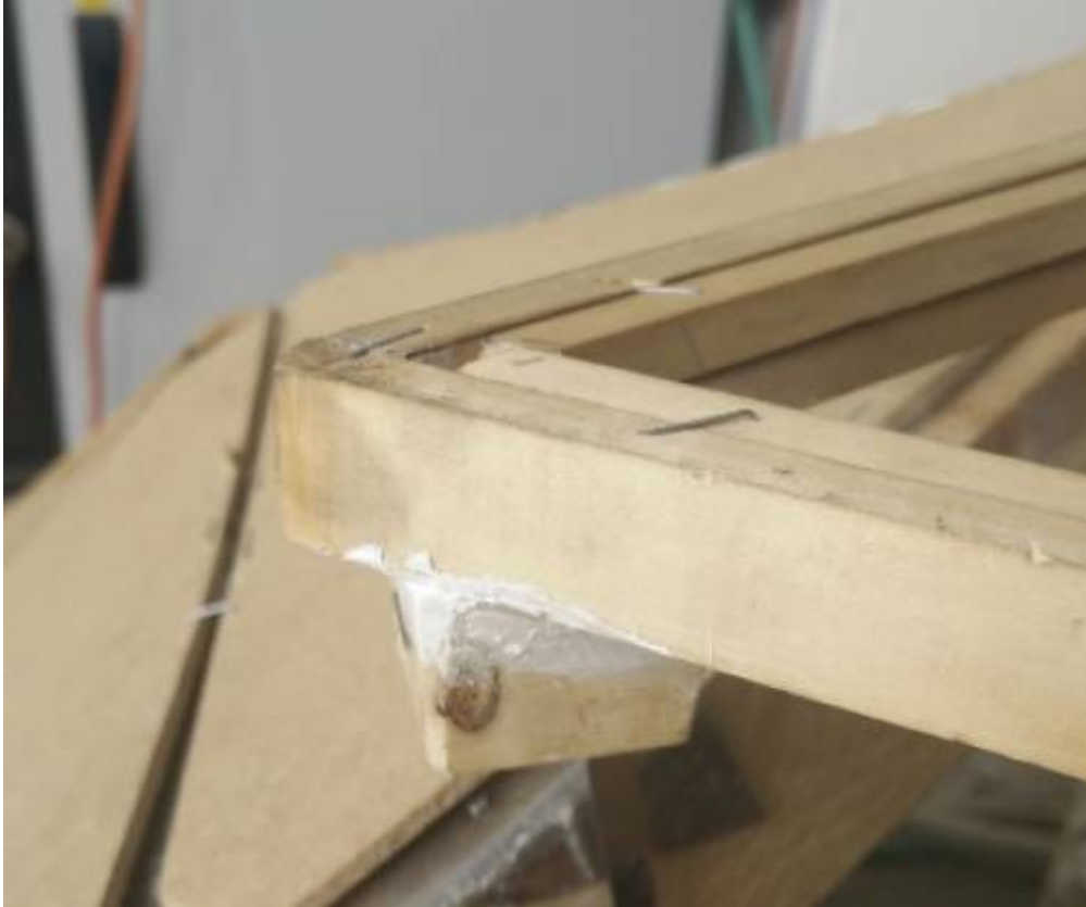
Figure 80: Wooden block to connect the arm of the servomotor to the window
