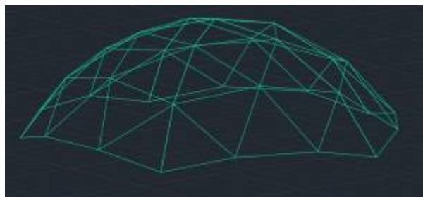
Figure 39: Beams of the top part of the dome
