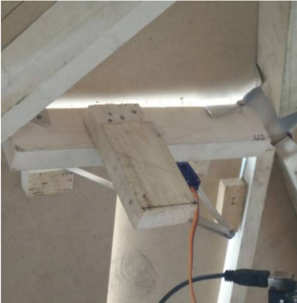
Figure 85: Wooden block to attach the servomotor
