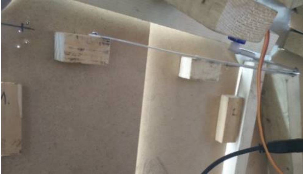
Figure 83: Connection of the arms of the servomotor
