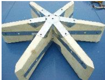
Figure 10: Straps for reinforcement Dome kits, 2016 [10]
