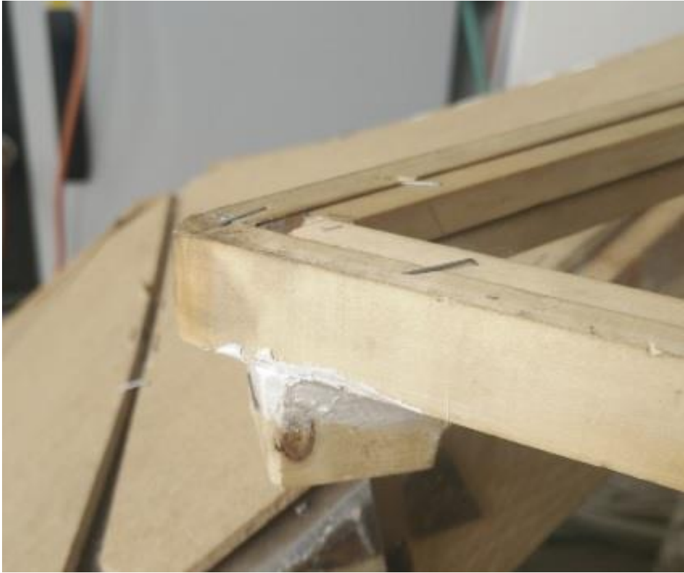
Figure 78: Wooden block to connect the arm of the servomotor to the window
