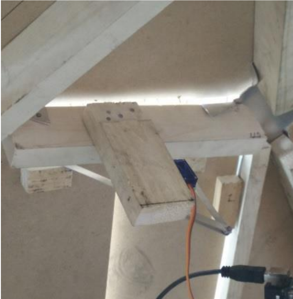
Figure 83: Wooden block to attach the servomotor
