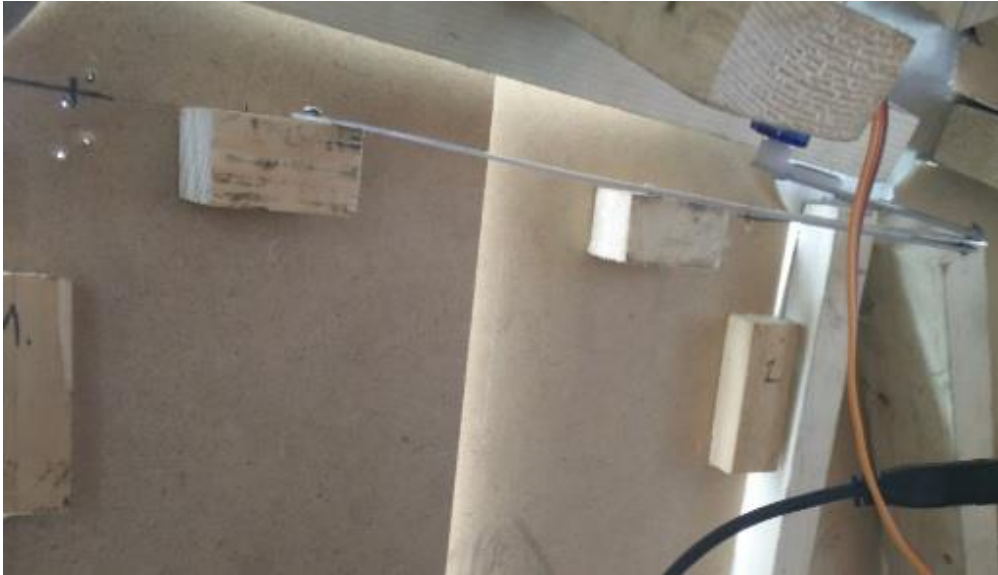
Figure 81: Connection of the arms of the servomotor
